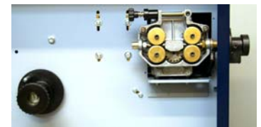
WIRE FEEDER INSIDE THE GENERATOR
